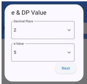
1. **Decimal Place:** In the dialog box, you can adjust the decimal places for weight precision. For example, if the weight is currently displayed as 2.00 and you want more precision, you can set the decimal to 3, displaying the weight as 2.000. This setting allows customization of decimal places according to your needs (e.g., 2.0, 2.00, 2.000, etc.).
